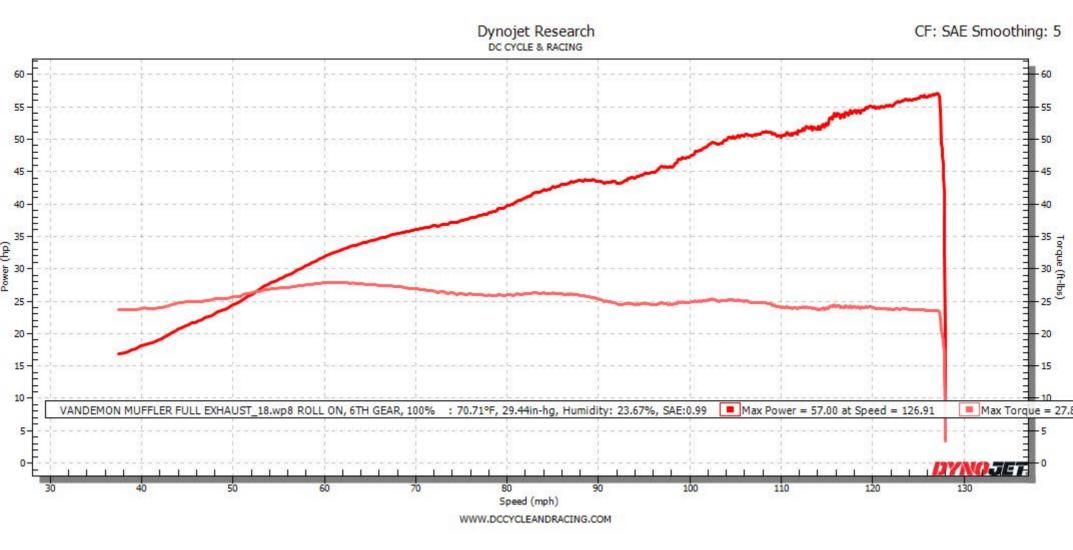
VANDEMON MUFFLER FULL EXHAUST\_18.wp8 [At: 4:46:18 PM, Wednesday, March 27, 2024] [Title: ROLL ON, 6TH GEAR, 100%] [As tested on Dynojet Model 250iX] [CF: SAE 0.99] [RPM: Inductive 1] [AFR Source: Dual WB2] Notes: FULL EXHAUST, DC TUNE
