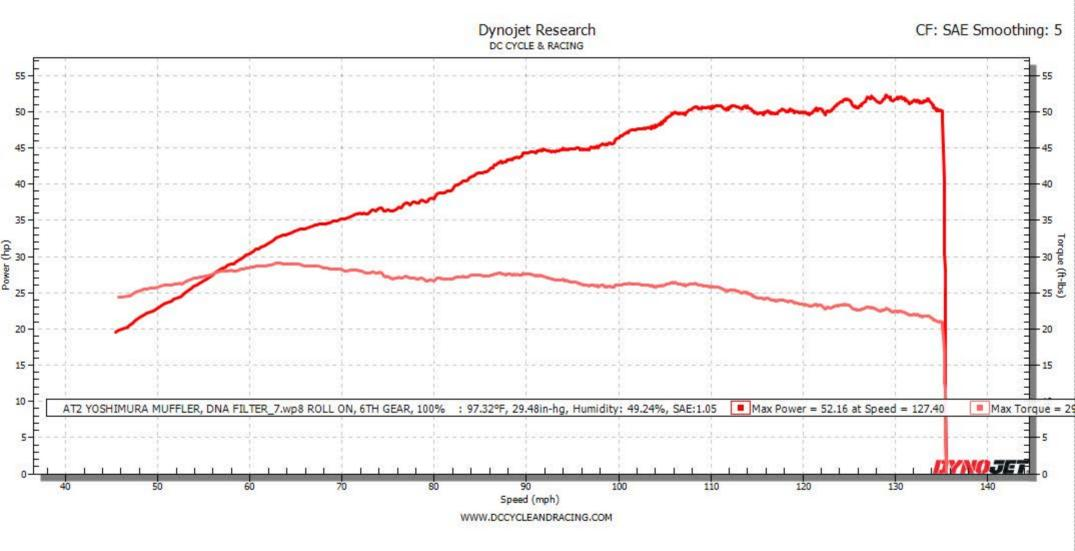
AT2 YOSHIMURA MUFFLER, DNA FILTER\_7.wp8 [At: 11:40:21 AM, Monday, July 29, 2024] [Title: ROLL ON, 6TH GEAR, 100%] [As tested on Dynojet Model 250iX] [CF: SAE 1.05] [RPM: Inductive 1] [AFR Source: Dual WB2] Notes: 2024450SS WITH AT2 YOSHIMURA MUFFLER, DNA AIR FILTER WITH LID, DC TUNE
