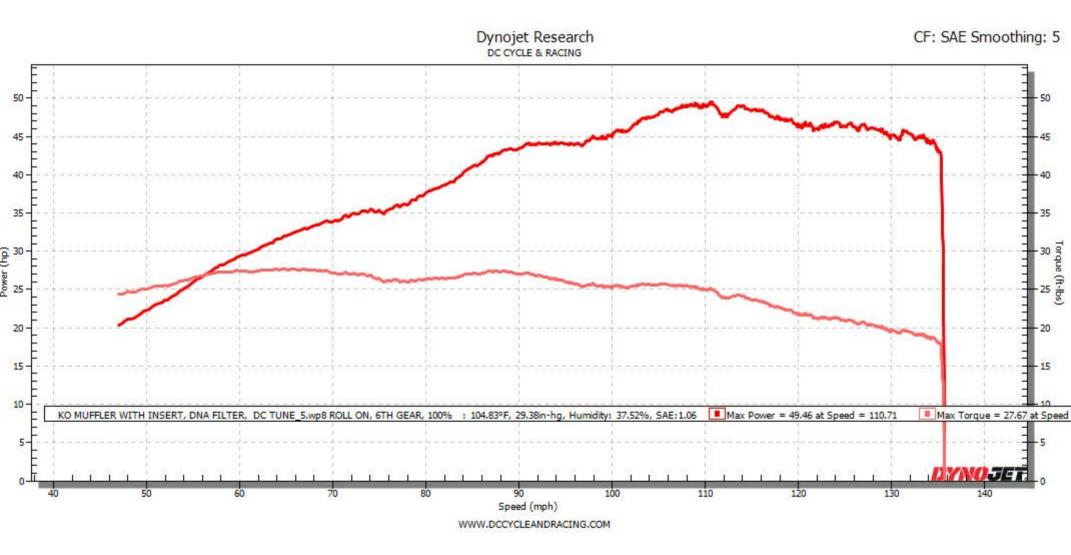
KO MUFFLER WITH INSERT, DNA FILTER, DC TUNE\_5.wp8 [At: 4:11:32 PM, Monday, July 29, 2024] [Title: ROLL ON, 6TH GEAR, 100%] [As tested on Dynojet Model 250iX] [CF: SAE 1.06] [RPM: Inductive 1] [AFR Source: Dual WB2] Notes: 2024 450SS WITH KO MUFFLER WITH INSERT, DNA AIR FILTER, DC TUNE
