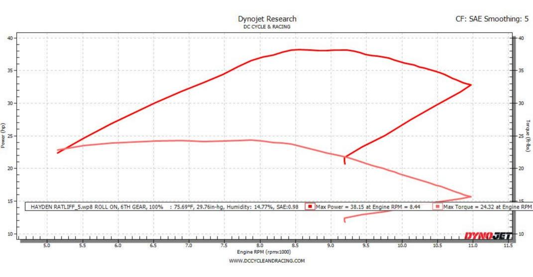
HAYDEN RATLIFF\_5.wp8 [At: 2:05:31 PM, Saturday, January 25, 2025 ] [Title: ROLL ON, 6TH GEAR, 100%] [As tested on Dynojet Model 250iX ] [CF: SAE 0.98 ] [RPM: Inductive 1 ] [AFR Source: Dual WB2 ] Notes: 2020 YFZ-450 ATV, MOTOR WORK, RECLUSE CLUTCH, FMF CARBON FULL EXHAUST, VORTEX ECU, BASE RUN
