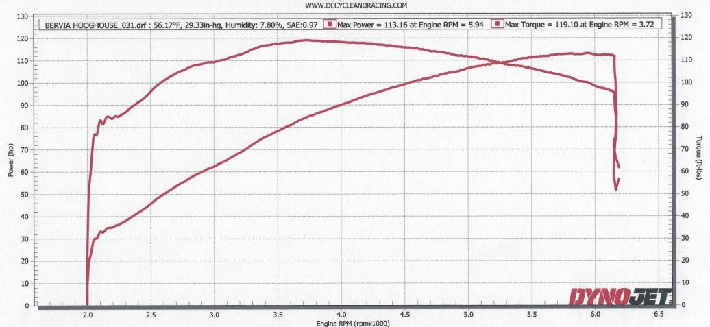
BERVIA HOOGHOUSE\_031.drf [ At: 7:44:37 PM, Tuesday, May 03, 2016 ] [ CF: SAE 0.97 ] [Title: 2000 ULTRA CLASSIC ROLL ON, 100%, 5TH GEAR] Notes: VIN 47954, MIL 23800 HORSE POWER INC THROTTLE BODY, BAKER 6 SPEED TRANS, SLIP ON MUFFLERS, DIRECT LINK TUNER, V111 S&S ENGINE TUNED BY DC CYCLE & RACING (DAVID CRANE)
